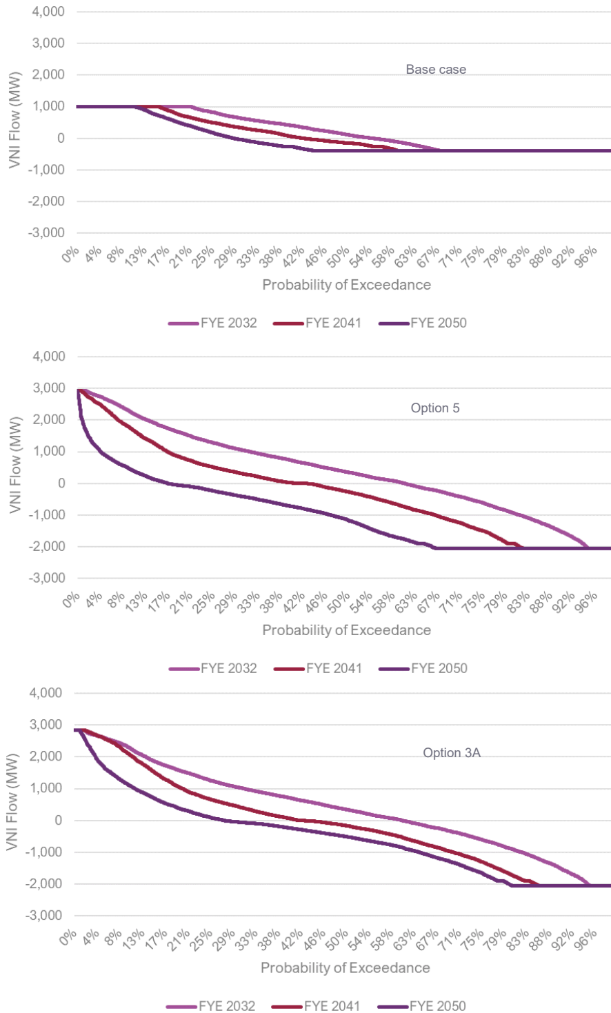
Figure 12 Flow duration curve – base case (top), Option 5 (centre) and Option 3A (bottom)
