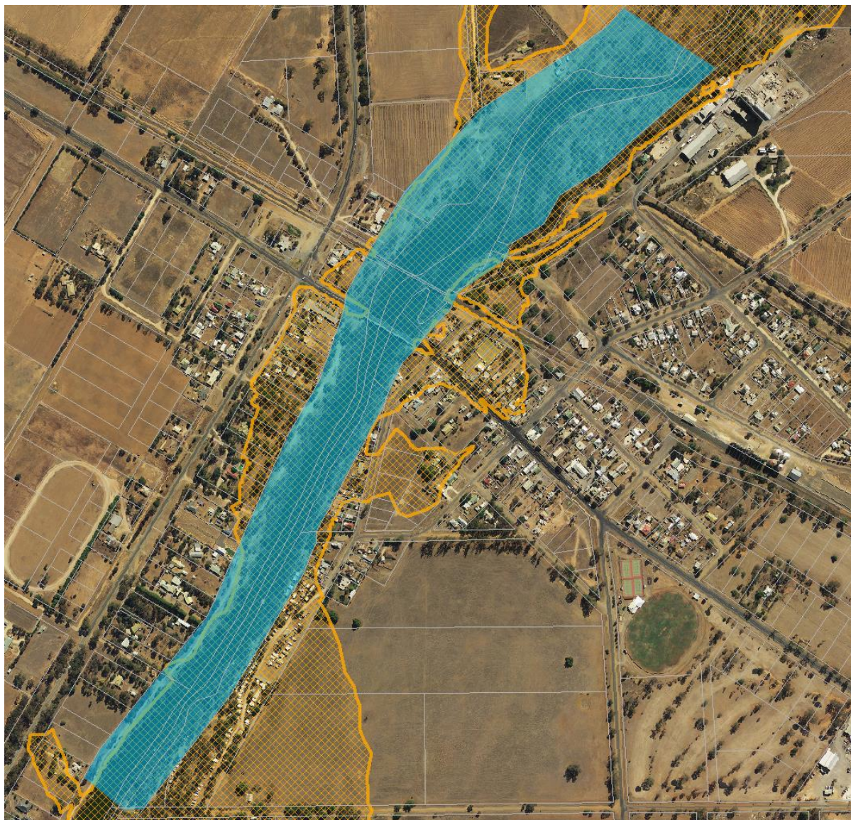
Figure 1 – Comparison of existing FO (Blue) and proposed draft FO (Orange hatched). Note: this map excludes existing and proposed LSIO i.e. the full flood extent is larger than this (see Figure 3).
